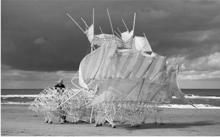
FIGURE 5.10 Theo Jansen with the strandbeest Plaudens Vela , which means flapping sails. The animal had a lot of sails so that it could move forward even in gentle breezes.
