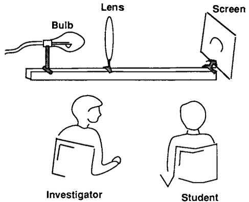
FIG. 1.3. Investigator asks student: "Suppose I were to cover the top part of the lens, leaving the bottom half uncovered. Would anything change on the screen?" The table shows the percentage of students who gave the correct answer both before and after instruction (Goldberg & McDermott, 1987).
