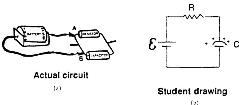
FIG. 1.5. (a) An actual circuit shown to a student during an individual interview; (b) Circuit diagram drawn by the student, who ignores the wire  $AB$  that connects the resistor and capacitor across the battery (Fredette & Clement, 1981).
